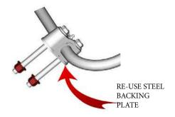
REMOVE THE BOTTOM BUSHING FROM THE BRACKET AND COAT THE INSIDE OF THE BUSHING HALVES WITH THE SUPPLIED GREASE.
